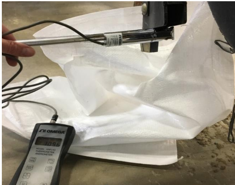
Figure 6. Air speed measurement taken prior to treatment repetitions.
