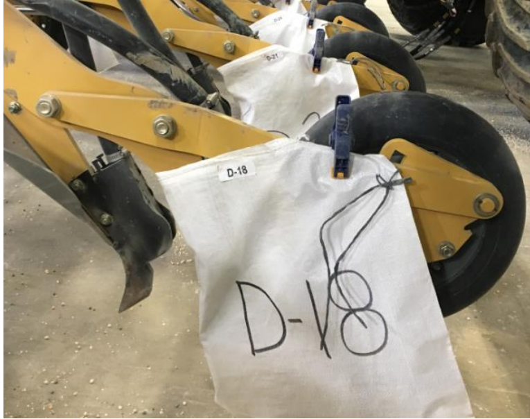
Figure 7. A collection bag fastened to the rear seed opener with clamp.
