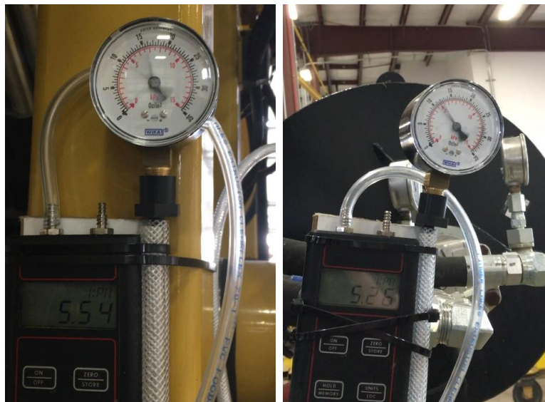
Figure 8. Static pressure measurements were taken before and during tests.
